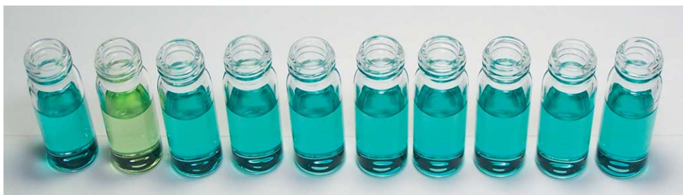
Figure 8. Color of the sensing ensemble (25 \mu\text{M} ) in the absence and presence of amino acids (25 \mu\text{M} ): from left to right; the sensor only, and the sensor with Cys, Glu, Asp, His, Lys, Arg, Gly, Val and Ser.
