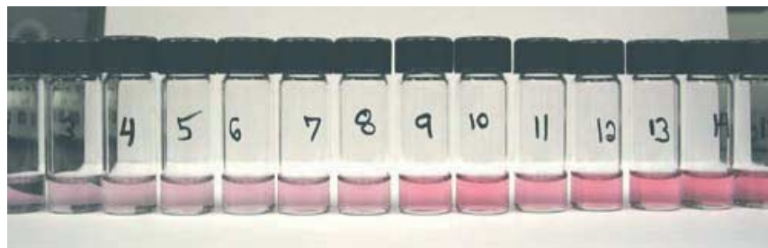
Figure 7. Color change observed in the presence of varying concentrations of uranyl acetate. The solutions in question have an isoamethyrin concentration of 1.686 \times 10^{-5} M and contain 4 equiv of \text{Et}_3\text{N} ; they were made up in methanol–dichloromethane 95:5 (v/v). The vials were stored in the dark for 9 days before the photo. The uranyl cation concentrations in the vials shown, labeled 4, 5, 6, 7, 8, 9, 10, 11, 12, 13, and 14, were 4.34 \times 10^{-6} , 6.06 \times 10^{-6} , 8.64 \times 10^{-6} , 1.12 \times 10^{-5} , 1.63 \times 10^{-5} , 2.13 \times 10^{-5} , 2.75 \times 10^{-5} , 3.36 \times 10^{-5} , 4.16 \times 10^{-5} , 4.94 \times 10^{-5} and 6.09 \times 10^{-5} , respectively.
