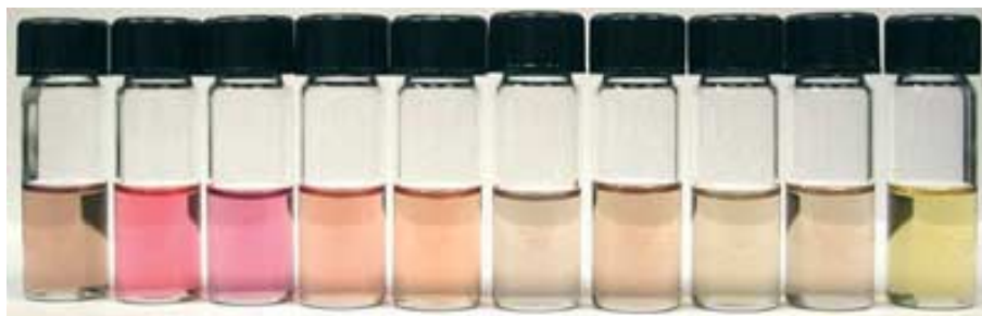
Figure 9. Colors of solutions of isoamethyrin ( 1.02 \times 10^{-4} M) containing 4 equiv of Et 3 N in a MeOH–CH 2 Cl 2 (95:5 v/v) solution. Far left: the acid salt of isoamethyrin and then from left to right after the addition of 2 equiv of, respectively, uranyl(VI) acetate, copper(II) nitrate, gadolinium(III) acetate, zinc(II) acetate, nickel(II) acetate, lead(IV) tetraacetate, manganese(II) acetylacacetate, and cadmium(II) nitrate. The vial on the far right contains the free base form of isoamethyrin.
